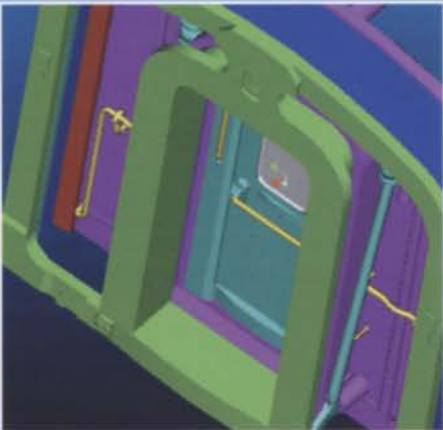
CAD drawing of newly designed, separately applied vestibule
