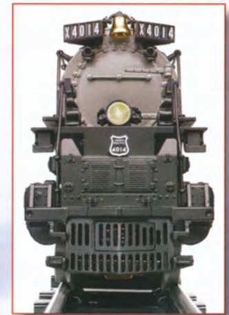
Prototypical pilot-mounted air brake radiators
