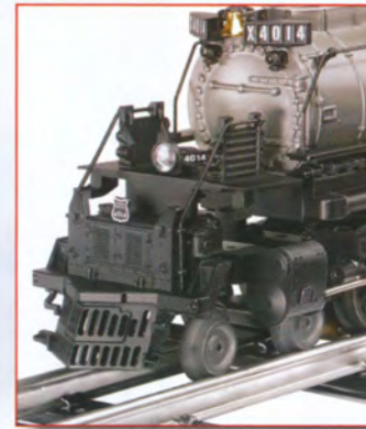
Prototypical pilot-mounted air brake radiators
