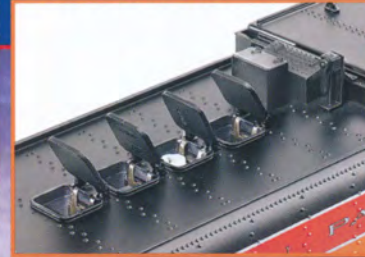
Opening tender water hatches reveal RailSounds controls
